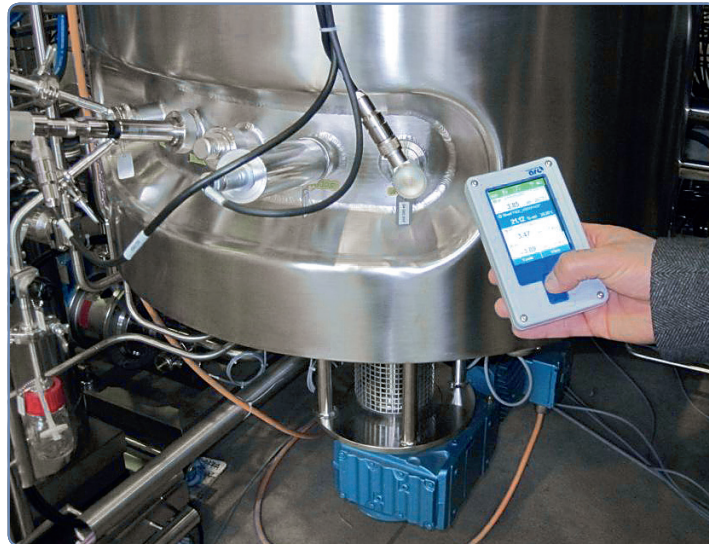
Figure 3: Arc sensor operation with Arc View Handheld at main fermenter
